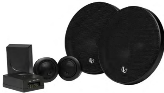
ALPHA 650C 6-1/2" (165mm) 2-Way component system speaker Power Handling: 45Wrms, 315W Peak @ 4 ohms Sensitivity ( @ 2.83V ): 91dB Frequency Response: 53Hz - 20kHz
